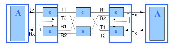
P.S: A=transmission equipment B=optical switch C=host cable D=standby cable
