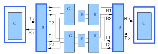
P.S: B=FSA C=transmission equipment G=relay station1 H=relay station2 E=host cable F=standby cable
