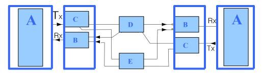
P.S: A=transmission equipment B=optical switch C=splitter D=host cable E=standby cable
