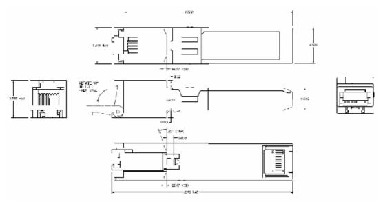
Figure 2. 3CP-RJ45-GE mechanical dimensions
